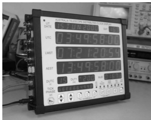
A prototype display unit for the Australia Telescope Distributed Clock.
