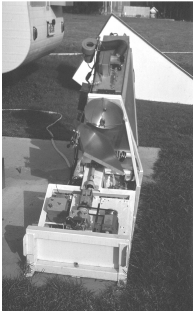
Figure 2: One of the interferometer antennas plus associated receiver electronics
