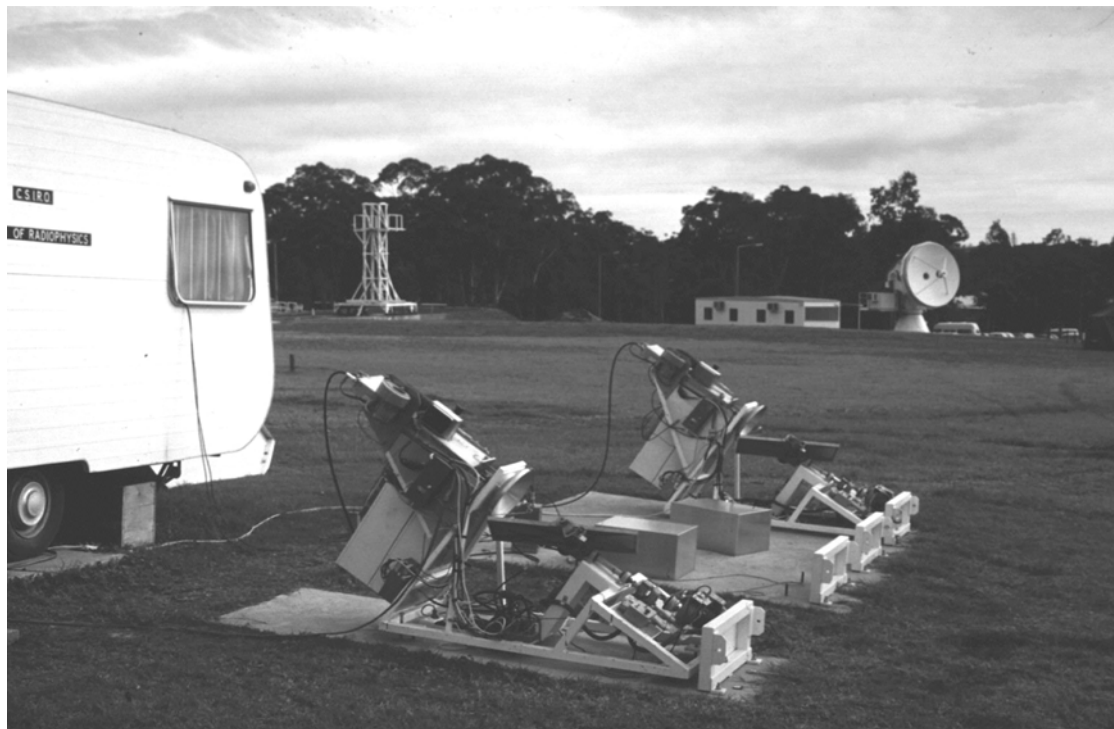
Figure 1: The 100-GHz interferometer with the 4-m telescope in the background
