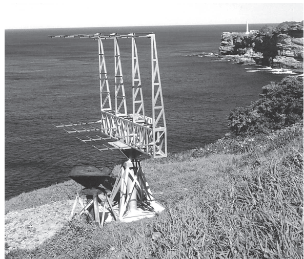
A full size replica of an 8-element Yagi array that was used at Dover Heights during 1951 – 1952. This was one of several Yagi arrays that were used on the site as a “sea interferometer”. In this technique, an interference pattern was recorded by combining radio waves detected directly from the source and from a reflection off the sea. The replica antenna has been installed on the cliff top next to the original mount, as a scientific memorial.
