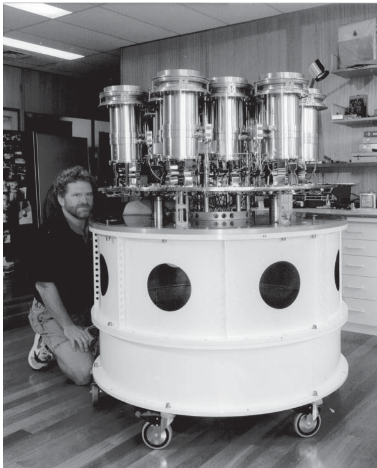
Pat Sykes with the Parkes 13-beam multibeam receiver ready for final assembly in the Marsfield cryogenic lab.
