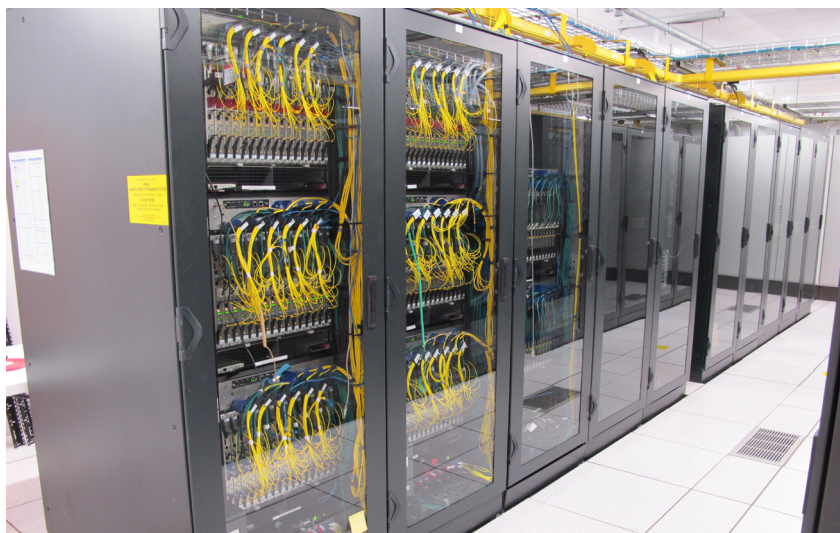
The new ASKAP hardware correlator, installed at the MRO.
