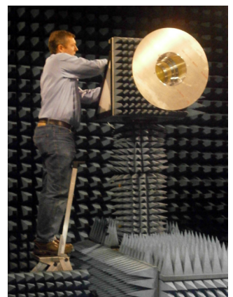
Measuring the feed pattern of the FAST test receiver in an anechoic chamber.
