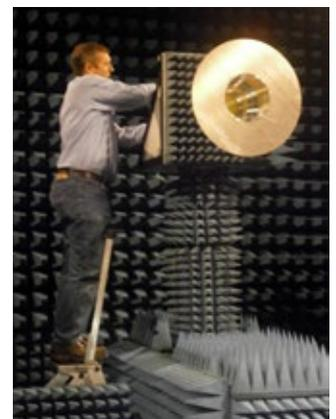
Measuring the feed pattern of the FAST test receiver in an anechoic chamber.
