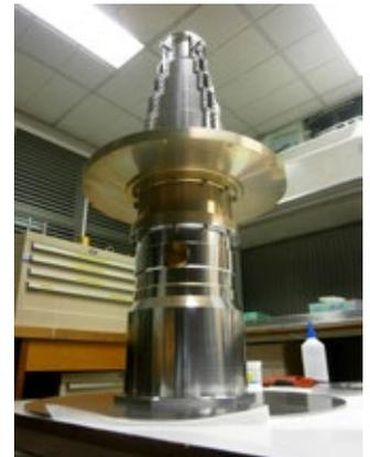
The input waveguide assembly for the FAST test receiver.
