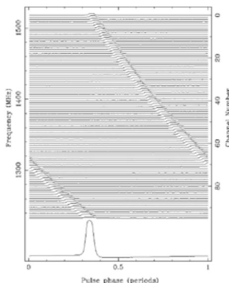
Figure 1: Pulse phase versus radio frequency ( $\nu$ ) for the strong, highly dispersed pulsar PSR B1641-45, recorded using one of the 96 x 3-MHz filterbanks built for the 20-cm Multibeam system. The dispersive delay is proportional to  $\nu^{-2}$ .
