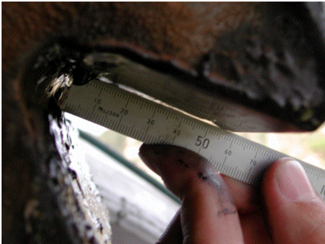
Fig 8: Wear on the rack teeth (still to be remedied).
