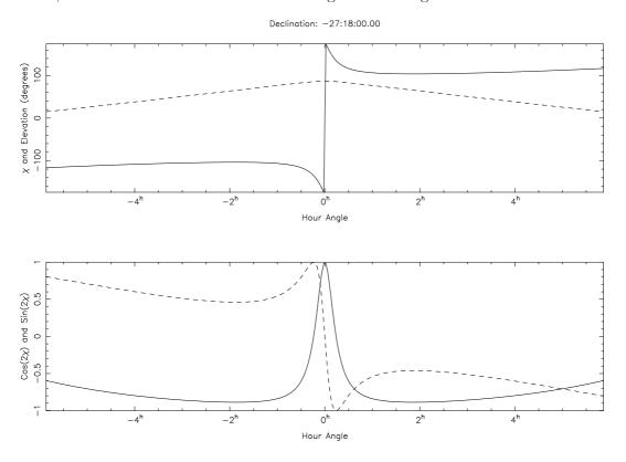
Figure 1: The parallactic angle  $\chi$ , elevation, and the functions  $cos(2\chi)$  and  $sin(2\chi)$  as a function of hour angle for the source PKS 1519–273, as plotted by PARAPLOT. Most of the variation in  $cos(2\chi)$  and  $sin(2\chi)$  occurs in the hour across transit.
