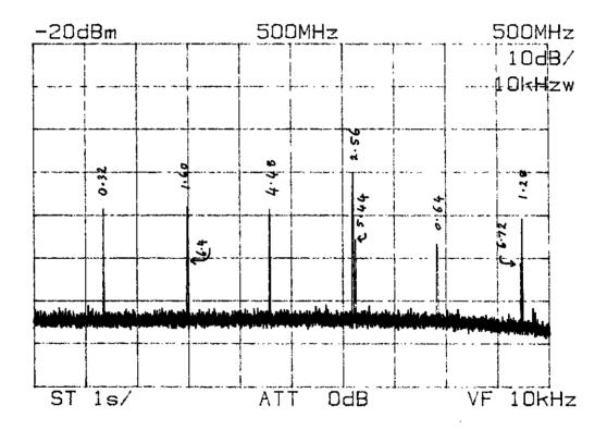
The leakage of the 160 MHz test signal from the RF port to the IF port was approximately -43 dB. All intermodulation products on the IF were at least 50 dB below the level of the test signal injected into LO port. This is a very good result. These mixers have excellect rejection of spurious signals on the LO port.
