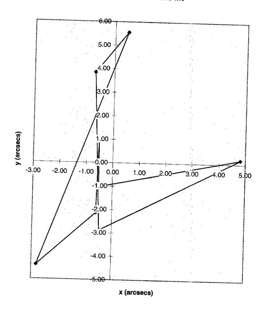
Figure 3: The polar wandering measured at the elevation bearing, after lifting the antenna
