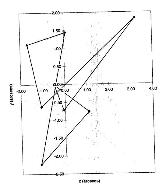
Figure 2: The polar wandering measured at the elevation bearing, before lifting the antenna
