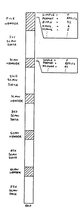
FIGURE 1: A TYPICAL RPFITS FILE STRUCTURE
