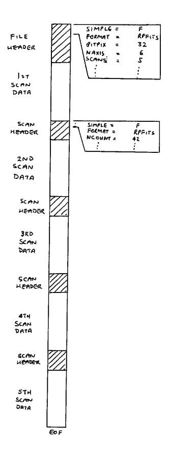
FIGURE 1: A TYPICAL RPFITS FILE STRUCTURE
