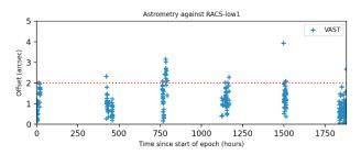
Figure 1: Plot showing average astrometric errors with respect to the RACS-low catalogue for a series of VAST epochs taken during full survey observations over the last few months. The offsets are usually less than the indicated 2" level, but poor weather conditions can cause more rapid departure from the phase solution of a given bandpass observation, leading to larger errors on occasion. Figure provided by Emil Lenc.
