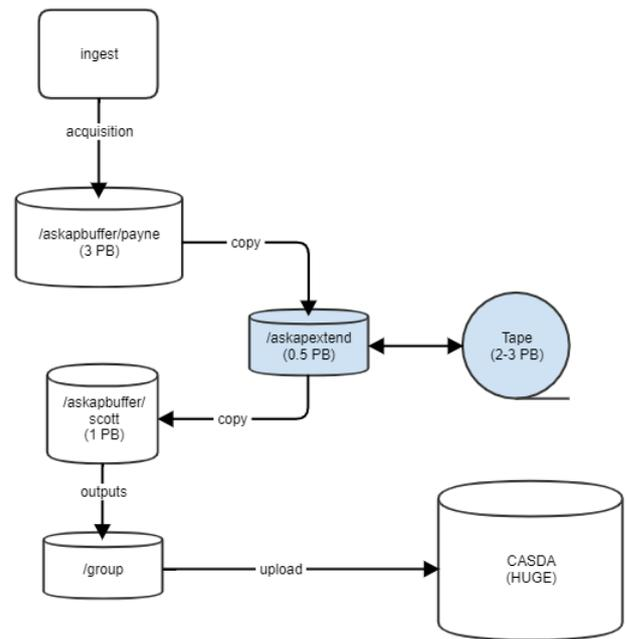
ASKAP data flow diagram highlighting the new tape stage
