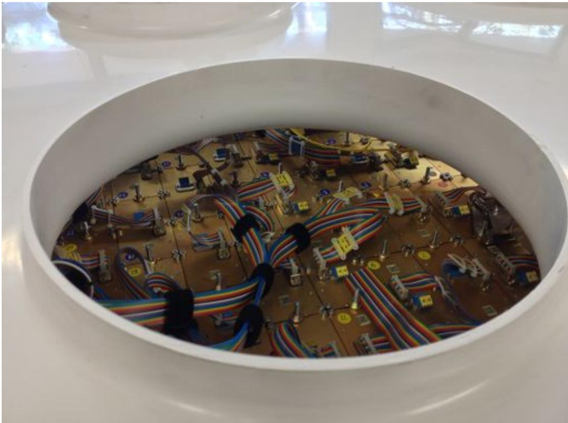
*Figure 2: Prototype Mk II phased array feed undergoing integration tests at the Marsfield labs.*
