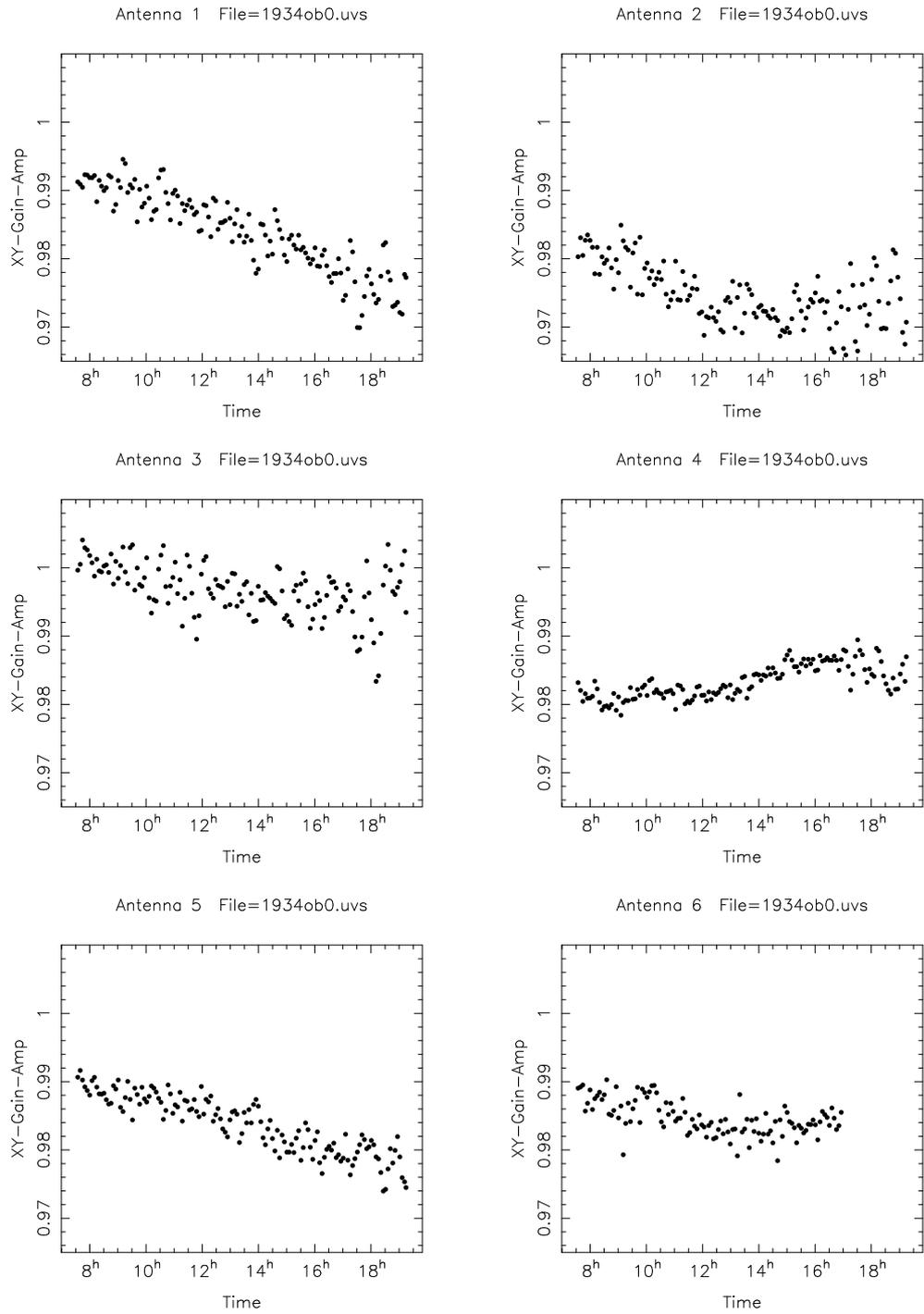
Figure 9: Ratio of antenna X and Y gain amplitudes as a function of time for the off-centre 1934-638 observation.
