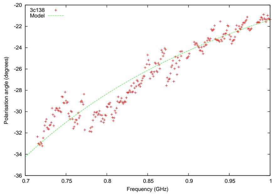
Figure 3: The measured polarisation angle of 3C138 as a function of frequency. The line gives the expected angle for a source with intrinsic polarisation angle of  $-9^\circ$  and  $RM = -2.4 \text{ rad/m}^2$ .
