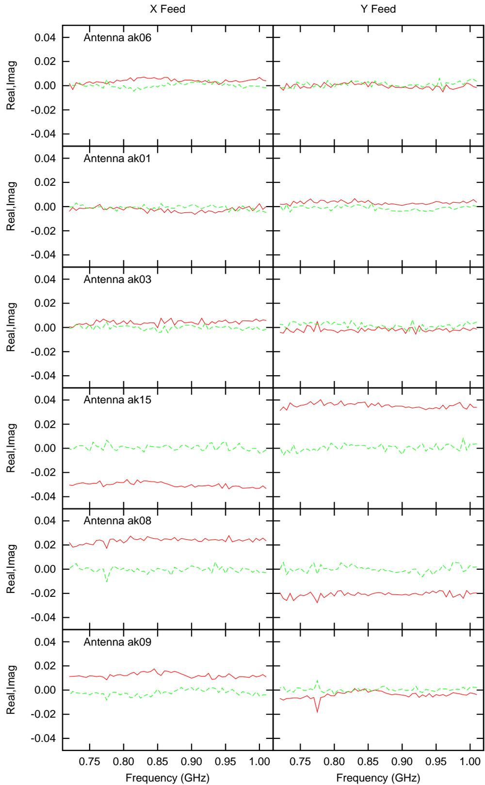
Figure 1: Polarisation leakage solutions for the six BETA antennas derived from 1934-638. Left and right columns are the X and Y feed solutions respectively. The real part is in red and imaginary in green.
