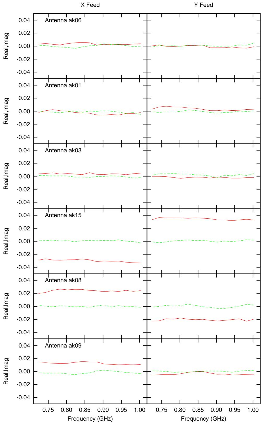
Figure 2: Polarisation leakage solutions as for Figure 1, but derived from 3C138. The poorer sensitivity of the observation led to coarser frequency resolution and noisier solutions.
