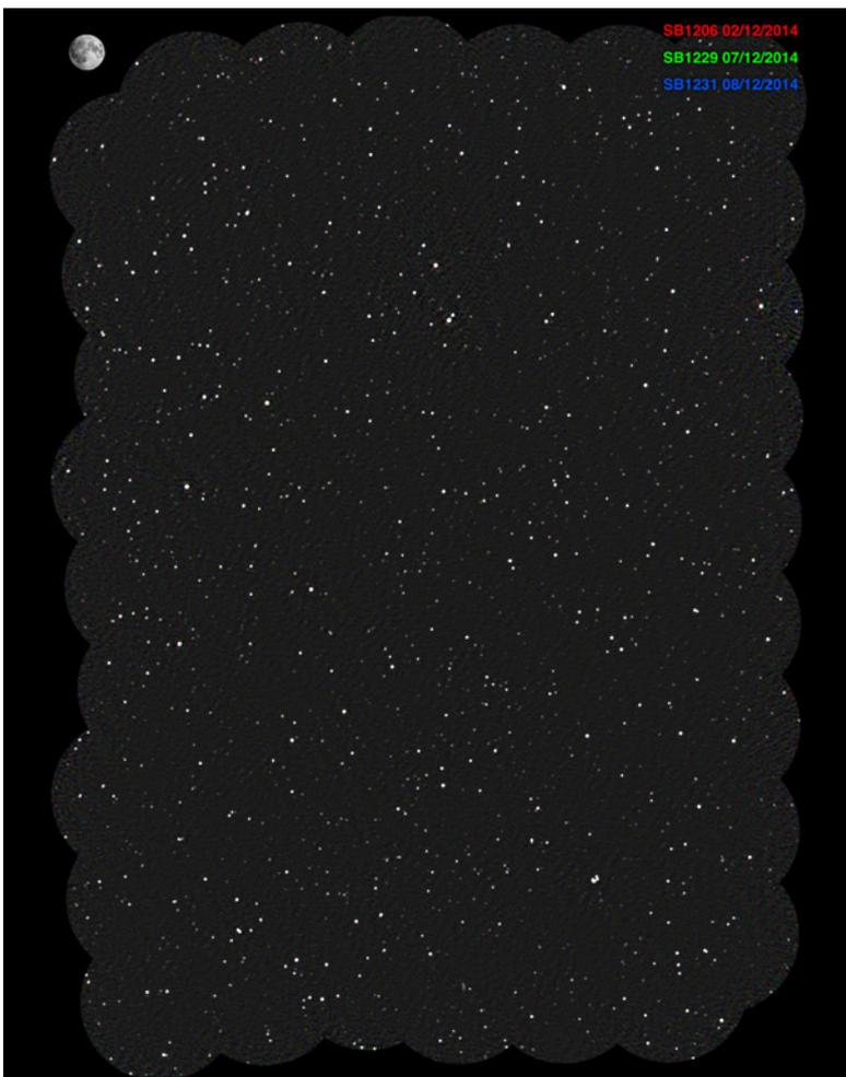
> A field in Tucana (Heywood, et al) imaged with BETA over 12 hours, covering 150 square degrees (an area approximately four times the size of the Southern Cross) and containing more than 2000 sources brighter than  $5\sigma$ . The image shows the rapid survey capability of the first generation PAFs and the stability of the system when performing wide-area surveys, highlighting the potential value of PAFs in studying variable sources.
