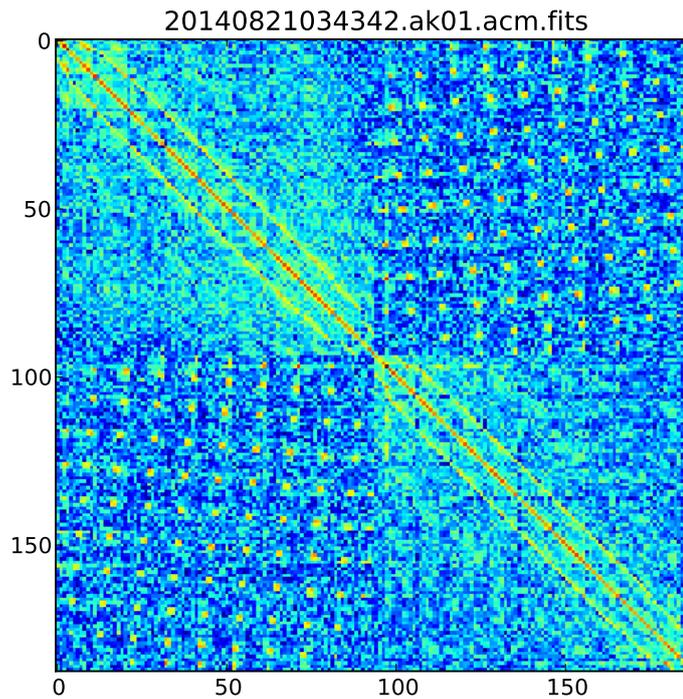
Figure 3.1: Amplitude (dB) of a typical ACM of 1 s duration, pointing at the SCP for a single 1 MHz channel near 850 MHz. The top-left and bottom-right quadrants show the co-polar XX and YY polarisations respectively, and the top-right and bottom left quadrants for the cross-polar XY and YX respectively. The three parallel diagonal lines in the co-polar quadrants are the autocorrelations and cross terms for which there is significant power (i.e. between adjacent co-polar elements).
