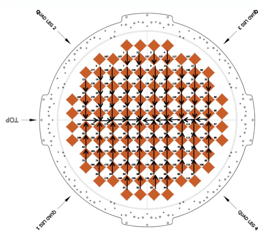
Figure 3.2: Routes taken to 'walk' from every X-polarisation port back to it's reference port (47 1-based). The route follows adjacent ports back to the centreline, and then along the centre-line to the reference port.
