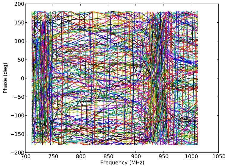
Figure 3.3: Phase spectrum of the ACM between each port, and its adjacent port for AK03 for the reference epoch. All ports show substantial phase structure, including a resonance around 950 MHz, many ports have intrinsic phase slopes.
