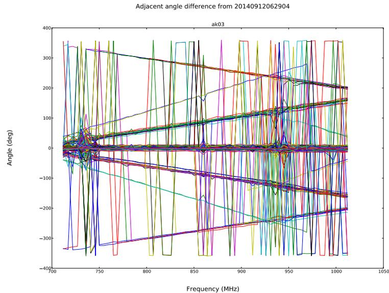
Figure 6.1: Phase spectrum of the ACM between each port, and its adjacent port for AK03 for an epoch, normalised by the reference epoch. Once the spectrum has been normalised, the phase structure disappears, and delay jumps are clearly visible.
