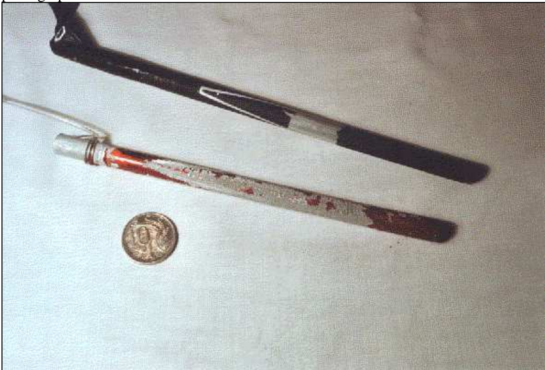
Figure 6 – Some failed etching attempts. The black coating is enamel paint, the red coating is photographic resist.
