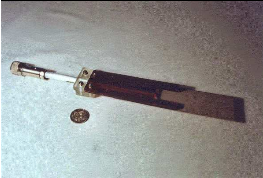
Figure 11. – The underside of the balun/taper. The shape of the bracket can be seen. Notice the gap at the point where the balun connects to the PCB.
