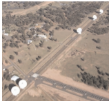
Figure 1: Recent aerial view of ATCA antenna array showing the 220-m north spur and the 3 km east-west rail track.
