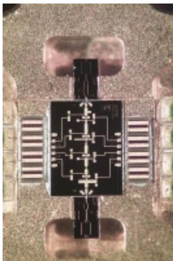
**Figure 4-2** *Early prototype 3.5 mm MMIC low-noise amplifier assembled in a waveguide mounting. The central integrated-circuit region is about 3 x 2 mm.*
