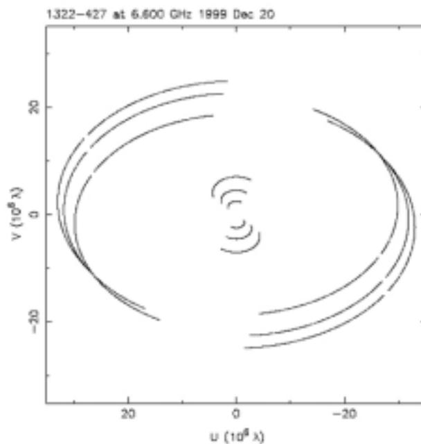
**Figure 4-7** *U-V plane coverage of the Australian VLBI network during December 1999 observations of Centaurus A at 6.6 GHz. The sweeping outer arcs are due to baselines from Ceduna to ATNF antennas at Narrabri, Mopra and Parkes. The addition of Ceduna improves substantially the imaging quality of the network.*
