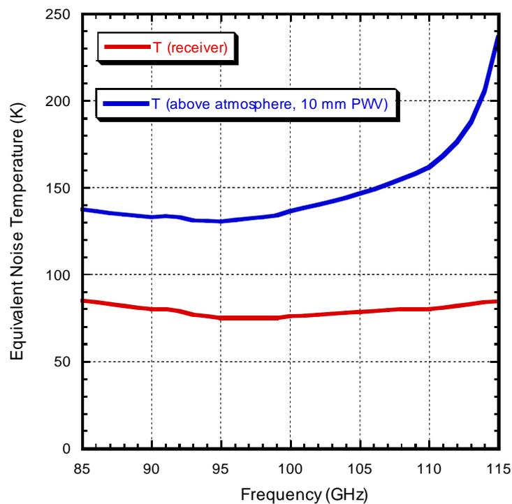
**Figure 4-1** Plots showing the expected variation in ATCA equivalent noise temperature as a function of frequency in the 12 and 3.5 mm bands. The red traces show the receiver (flange) noise temperatures, while the blue lines show indicative above-atmosphere system temperatures with 10 mm of precipitable atmospheric water-vapour - a common value during Narrabri winters.
