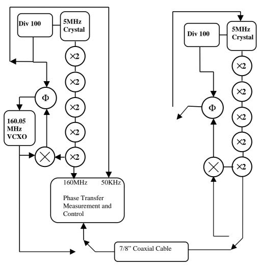
A 160.05MHz signal is derived from a stable reference Crystal at the central site using an offset phase locked loop. A 50kHz signal is derived from the 5MHz central site crystal by a divide by 100 circuit. The 50KHz signal is used as a phase reference by the Phase Transfer System.
