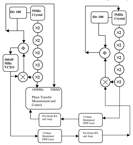
In stage 1 of the Local Oscillator upgrade a pair of Compact Array antennae will be fitted out with fibre optics to distribute the 160,05MHz signal produced at the central site. Antenna CA06 is currently similarly equipped. This stage will also field trail fibre optic connectors and components by selectively cabling some of the existing stations and the new array stations.
