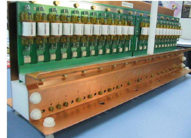
RF switch and capacitor for tuning the probe coil.
