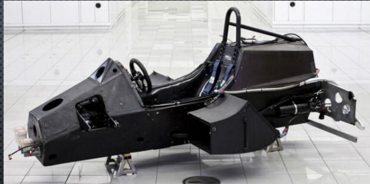
Survival cell monocoque
