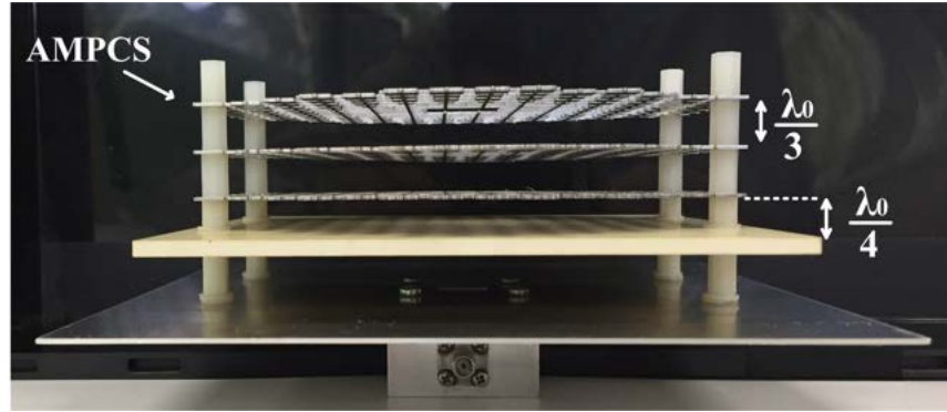
Figure 5.6: A prototype of the fabricated AMPCS loaded on the ERA. The AMPCS and the PRS are made of thin sheets of stainless steel, and Rogers TMM4, respectively.
