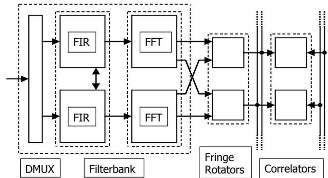
**Figure 2** Basic Filterbank Correlator Structure
