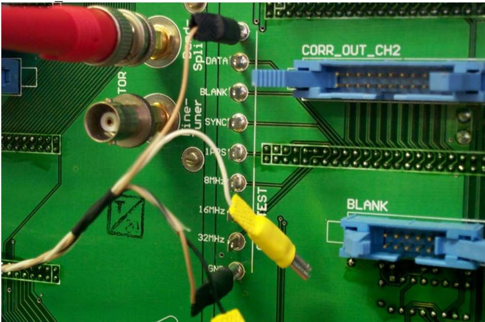
4. Next connect the yellow socket with the black wire to the 32MHz test pin.
