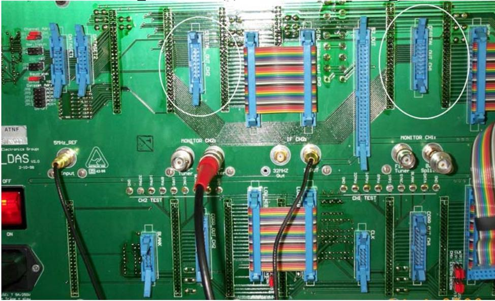
2. Open the latches of the DIGITAL\_OUT port halfway.
