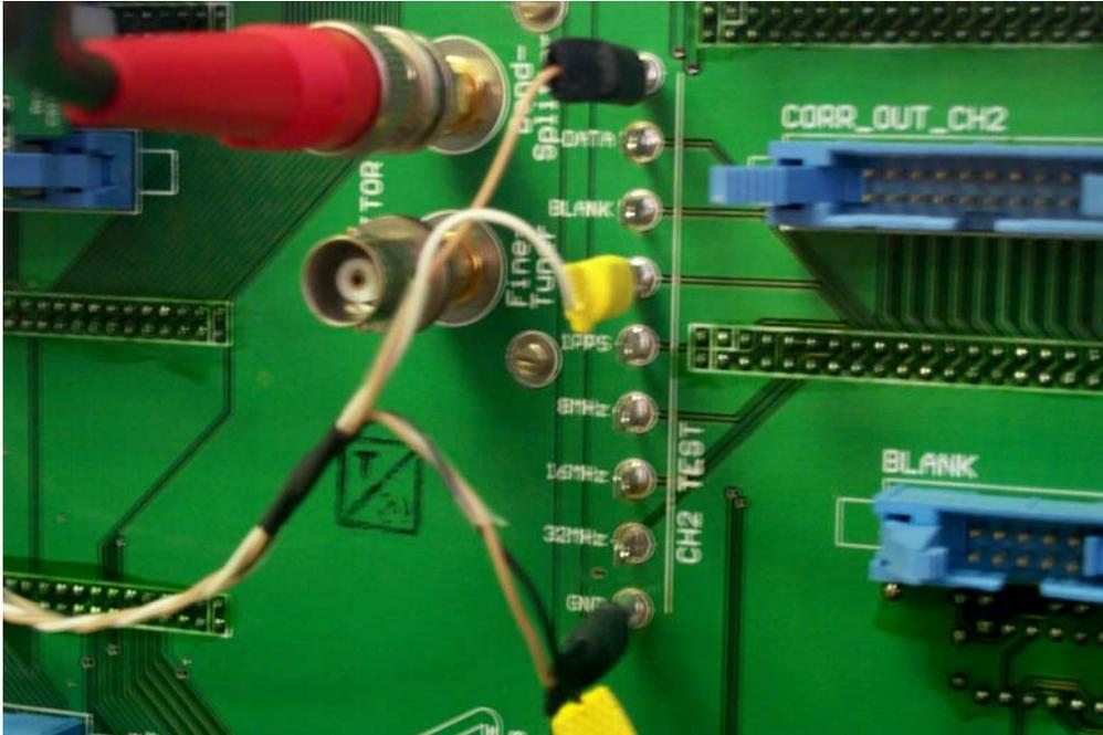
5. Next connect the yellow socket with the white wire to the SYNC test pin.
