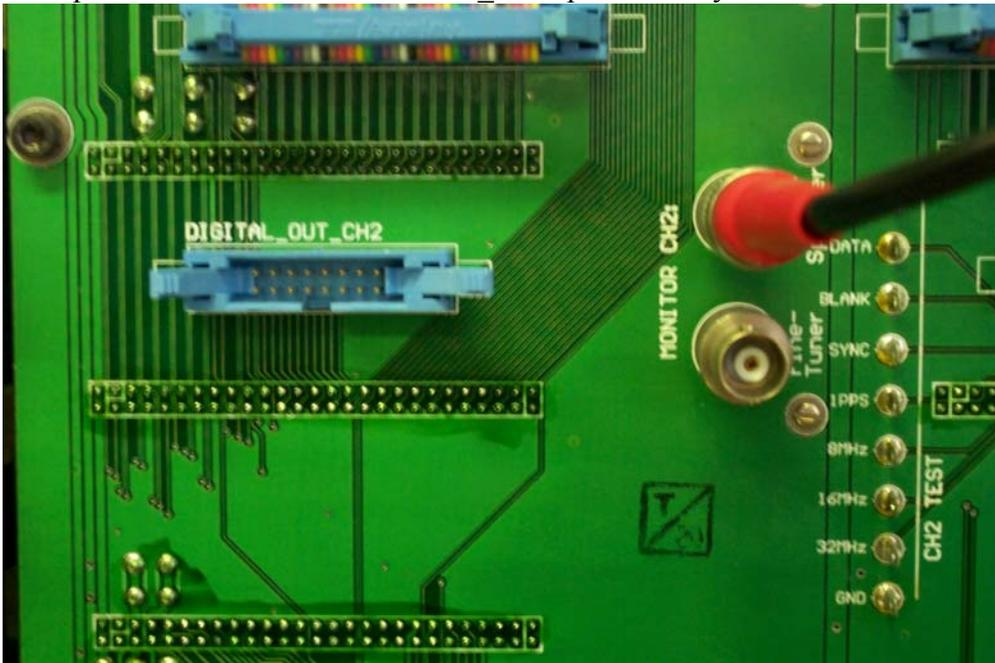
3. Push the 16 Way socket on the bottom of the Dig\_Out board into the DIGITAL\_OUT Port.
