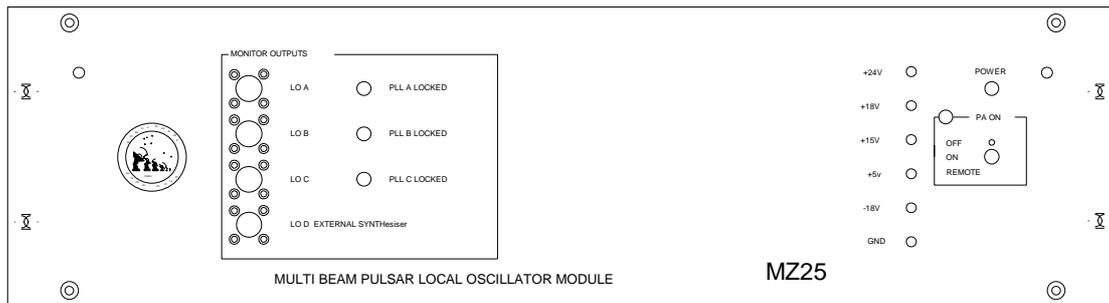
Test points for the D.C supplies are available on the front panel.
