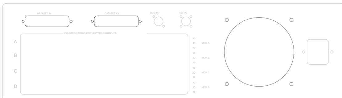
The station clock is connected to the RF IN BNC connector on the rear panel. The station clock can be either 5 or 10 MHz depending on the setting of links in the internal synthesisers. The Reference level should be +3dBm to -3dBm.
