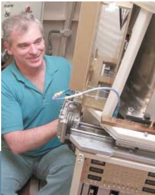
Les Reilly, a member of the ATNF receiver group, working on a newly installed millimetre-wave receiver package.
