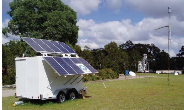
The remotely operating radio-frequency monitoring set-up to be deployed at Mileura Station during 2005. Note the antenna mount on the right as well as the solar-powered radio-frequency-screened trailer containing the data collection equipment.
