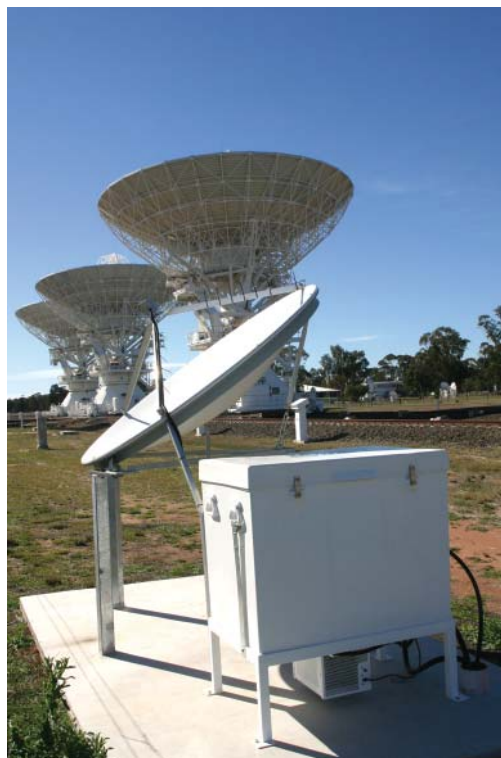
One of the two stations used for the atmospheric seeing monitor. Three of the Compact Array antennas can be seen in the background.
