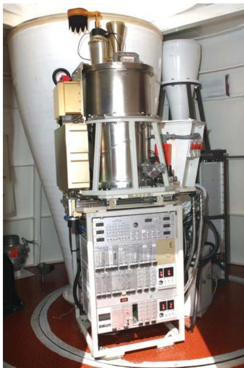
A newly-installed 3-mm system on one of the Compact Array antennas. The feed horn for observations at 3 mm is seen in front of the much larger feed horn used for observations at 20 cm.
