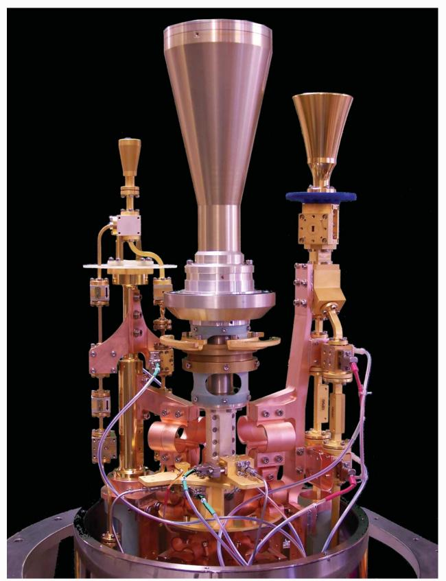
A Compact Array mm-wave receiver with prototype 7-mm components. From left to right are signal paths for 3-, 12- and 7-mm wavelength bands respectively. The majority of components are cooled to cryogenic temperatures through connection to a closed cycle helium refrigerator via the elegant copper metalwork. This minimises thermal noise that might otherwise mask the astronomical signal.
