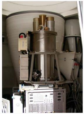
The mm-wave receiver with a prototype 7-mm system included mounted in the turret of Compact Array antenna 6.
