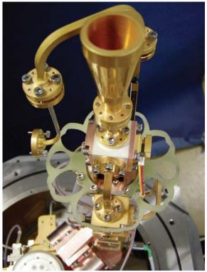
Feed and calibration signal waveguide of the mm-wave package for the Mopra telescope.
