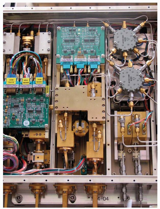
The millimetre receiver's complex, precisely engineered and modular conversion housing. Conversion modules make ready the amplified, high frequency astronomical signal from the receiver for processing by the ATNF's backend electronics. The modules, from left to right, function in the 3-, 7- and 12-mm wavelength bands respectively. Signal path components and control and monitor electronics are visible.
