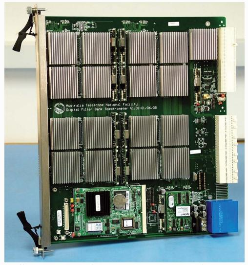
One of four signal processing boards for the Mopra spectrometer. The physical size of the board is approximately 40 cm x 40 cm. Photo: Evan Davis, CSIRO
