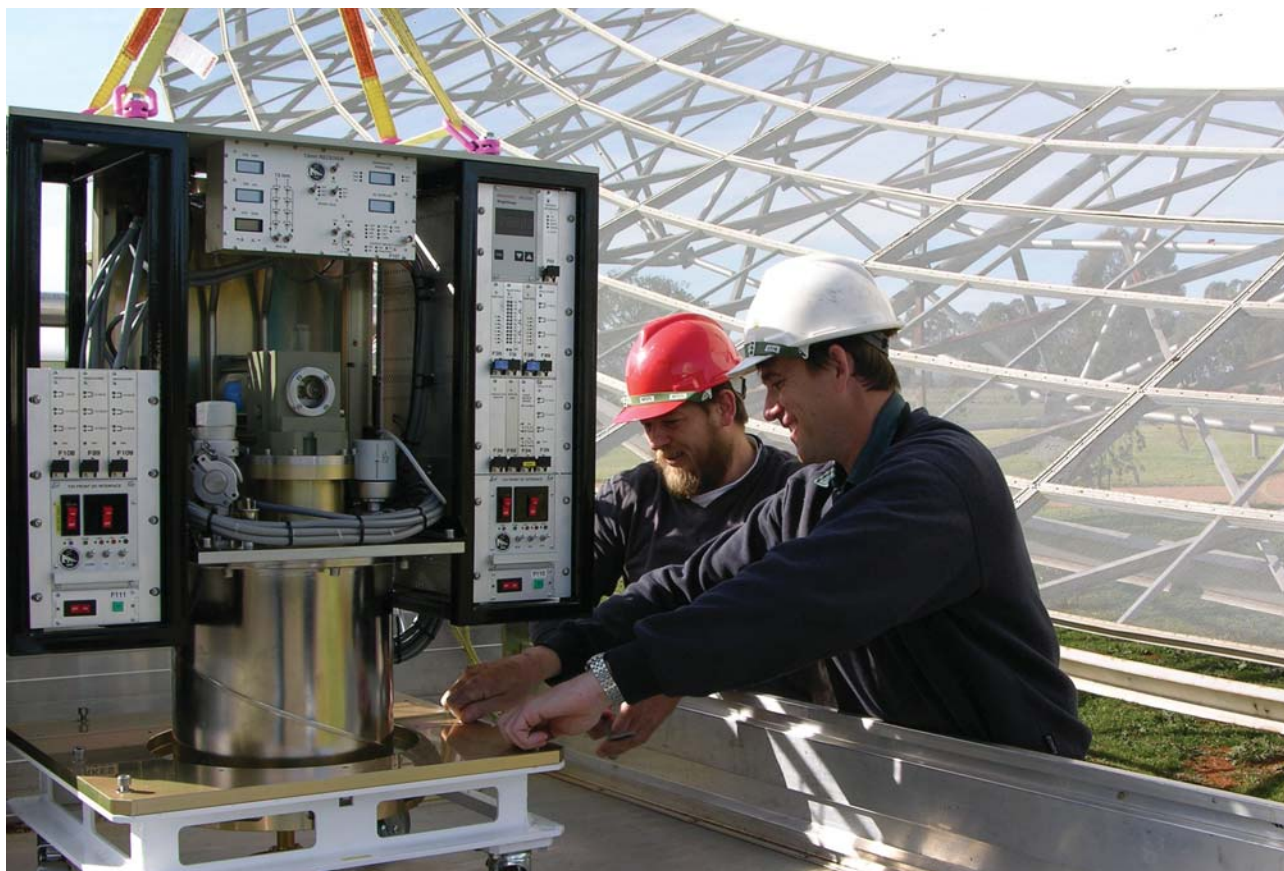
Mark Bowen and Ken Reeves during the installation of the new 13-mm (K-band) receiver at the Parkes telescope in September 2008. Credit: Henry Kanoniuk, CSIRO.
