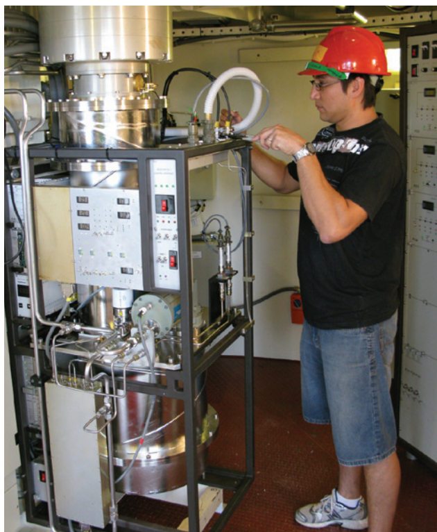
Santiago Castillo installing an upgraded 1.1 – 3 GHz receiver on a Compact Array antenna. Credit: Henry Kanoniuk, CSIRO.
