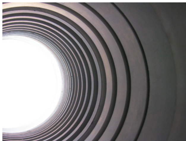
'Cold Sky View'; the interior of the ATCA CA-04 L-S feedhorn. Credit: Erik Lensson, CSIRO.
