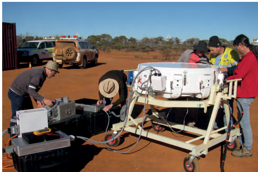
Staff at the Murchison Radio-astronomy Observatory preparing a prototype second-generation phased-array feed for ASKAP for testing.
