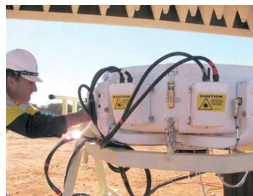
The set-up used for the ‘hot’ observation of an absorber box during ‘on ground’ tests of the prototype second-generation PAF at the MRO.
