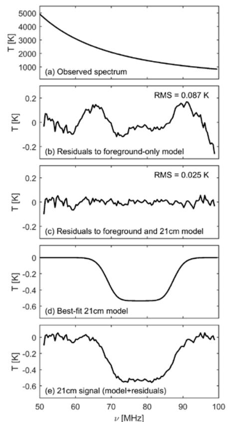
**Summary of the EDGES detection.** While the central frequency is in line with theoretical predictions, the peak amplitude is much greater and the absorption profile is unusually flat-bottomed. Image: Judd Bowman, Arizona State University.
