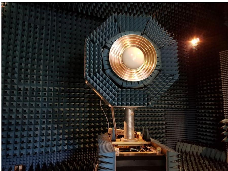
UWB-L in the testing facility confirming the design characteristics of high aperture efficiency, minimal ground noise pickup and no detectable resonances (which might otherwise be confused with spectral lines). Image: Santiago Castillo.
