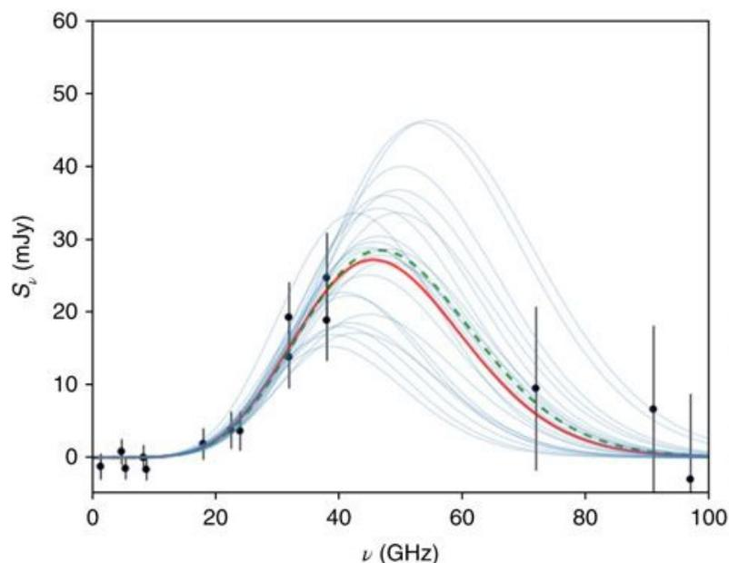
**Anomalous microwave emission from the MWC 297 system, with the modelled effects of dust and stellar wind subtracted. One data point was obtained with the GBT, the remainder with ATCA. The dashed line is the maximum likelihood fit and the solid line is the model. Thin lines are 24 samples drawn randomly from the posterior distribution. (From Greaves et al. 2018)**
