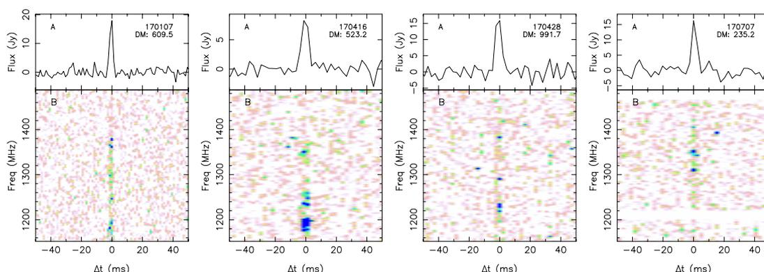
**Profiles (top panel) and dynamic spectra of a selection of ASKAP-detected FRBs. The spectra have been dedispersed to the maximum-likelihood dispersion measure. Flux densities reported in the pulse profile have not been corrected for off-axis attenuation. (From Shannon et al. (in press))**
