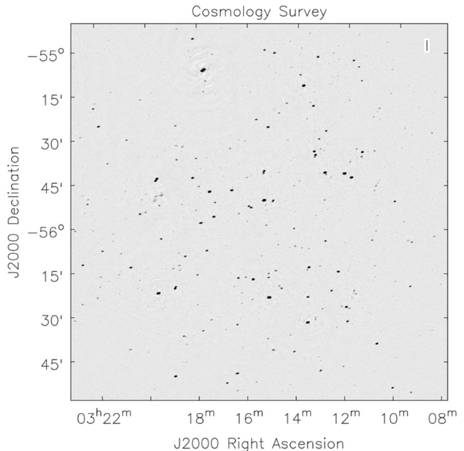
**Single beam image from one of the first observations from the largest survey to date (2000 square degrees). This image shows hundreds of radio sources, some with complex extended structure. (16 antennas, 240 MHz bandwidth, centre frequency of 912 MHz, 200 minutes per pointing).** Image: Aidan Hotan.
