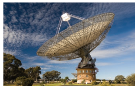
Parkes Radio Telescope Diameter 64 m Frequency range 0.7-26 GHz Bandwidths up to 1 GHz
