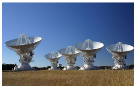
ATCA Collecting area 6 x 22 m Frequency range 1-105 GHz Bandwidth 4 GHz Configurable antenna location
