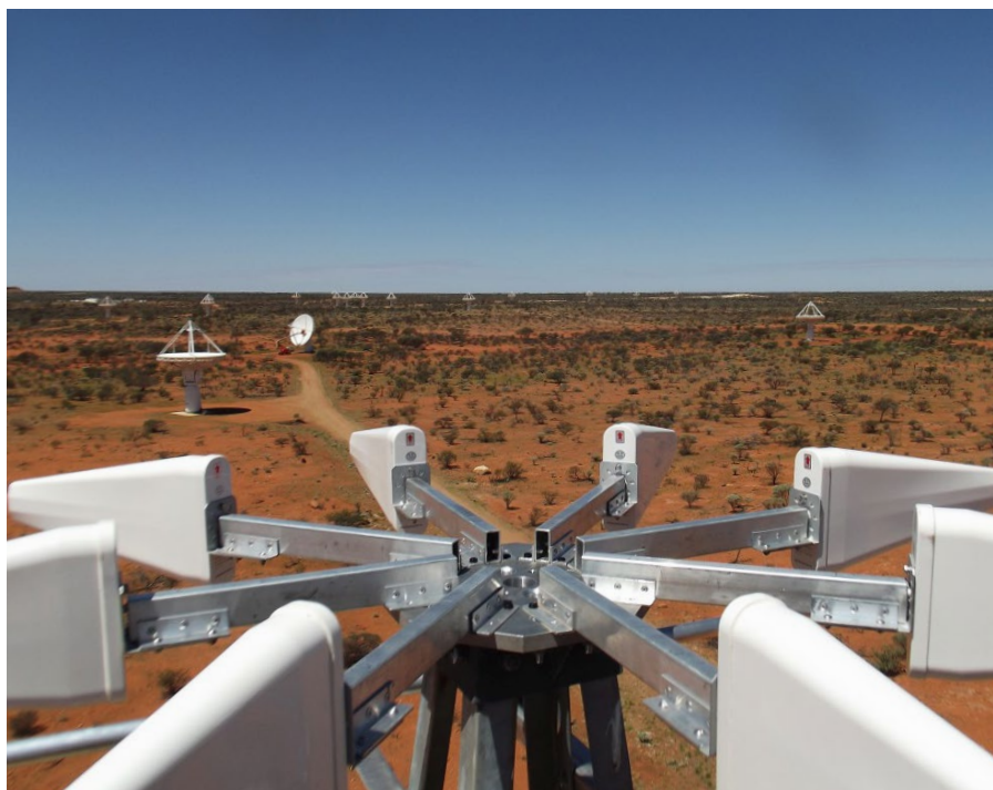
The RFI tower at the MRO monitors mobile phone signals and other interference occurring within and far outside the ARQZWA.
