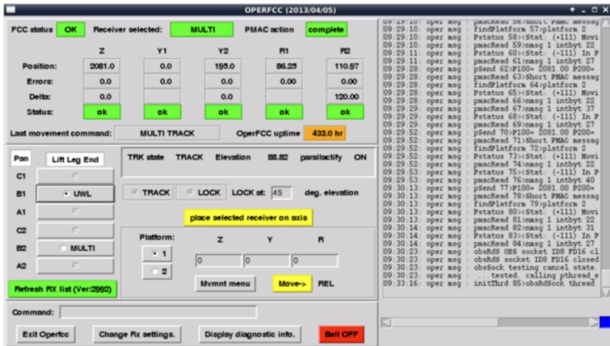
Your selected receiver will be on axis once all five status buttons are green and read 'ok'. Alternatively, you can turn on Focus cabin camera using Parkes Monitor & Control GUI to monitor the receiver change. Remember to turn the cameras off when the change is complete, as it is a source of RFI.
